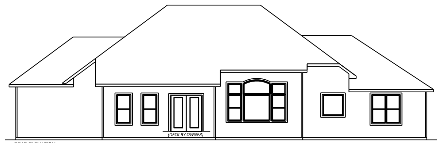
REAR ELEVATION 1/2 SCALE WINDOW/DOOR WRAP: 3.5" PLY-GEM
